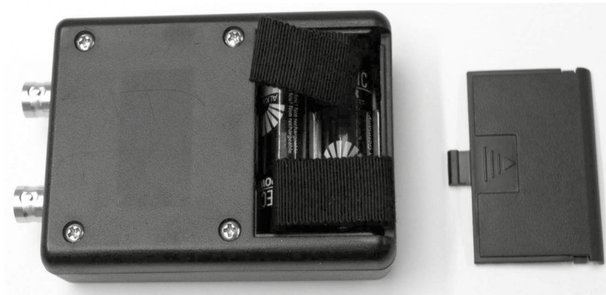
Fig. 3.1 Battery cover removed and battery compartment open: note polarity of batteries
