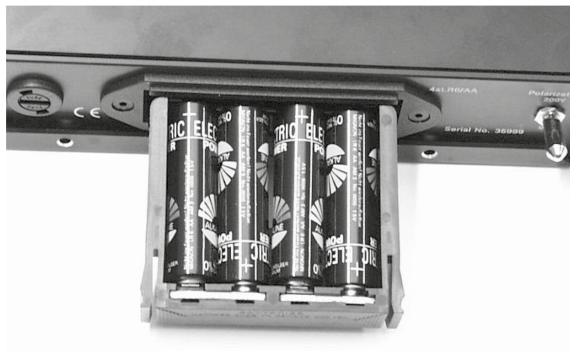
Fig. 3.1 Battery drawer open: note polarity of batteries
