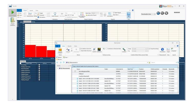
As soon as the drag&drop is finished, a new window will open in which the operator must tick-on the actual markers that are going to be used in the calculations. In the example below, data for the 'Washer' as well as the 'Background' are selected as correct data for the Receiving room as well as for the Background Noise.
