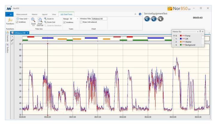
The General mode level profile with markers must be saved for later import to the Building Acoustic mode.
