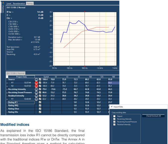
the Standard therefore gives a method for calculating modified indices based on an adaption factor which results in final indices that are closer to the traditional ones. This correction is based on an adaption term for each frequency band, and includes the total area of all boundary surfaces - named "Sb2" - in the receiving room.
