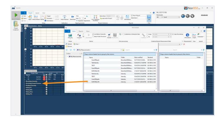
The induvial sub-areas may have varying sizes, and these values can be modified by the operator by opening the right-click menu on the sound intensity measurements displayed in the Project Data window. In this window, all the induvial sub-areas may be edited.
