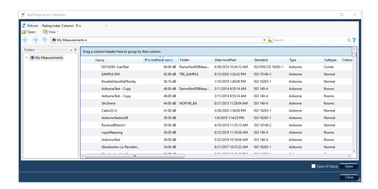
In the list of all available projects, a new column for the Rating Index is shown. Clicking on the column header will generate a filtering of all projects according to the selected rating index. The user may specify which rating index that are desired by opening the 'Rating Index Column' drop-down menu.
