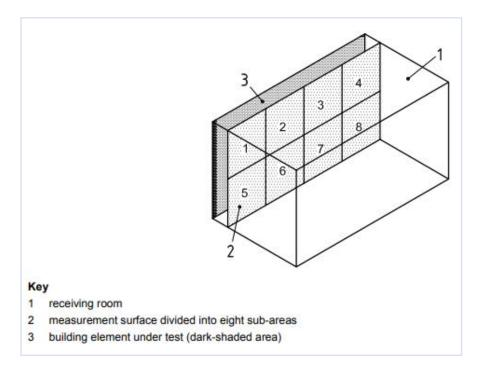
The second step is started by opening the Nor850 software in the Building Acoustic mode. Select the ISO 15186-2 Standard in the Rating menu, and key-in the receiving room volume and transmission wall area.
