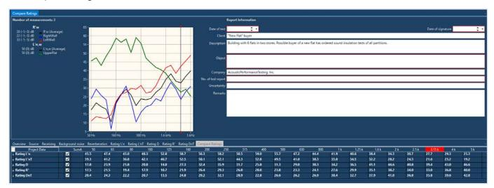
The type of rating index to be presented in this window is selected by clicking on the leftmost column in the lower part of the display. It is even possible to use Ctrl+Click to select multiple indices, or to limit the selection by opening the desired rating in the leftmost column and selecting only those of interest.
