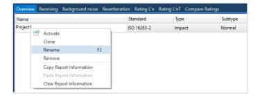
For setting up the second project, there are two possibilities. Either follow the same procedure from the Active Project window as for the first project, or use the Clone feature. The Clone feature is found in the right-click menu of the existing project in the Collection window. By selecting the Clone, a full copy of the first project is saved in the Collection with the extension "- Copy" on the previous name as shown in the example where the first project was named "Ceiling".
