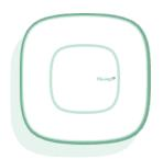
Wait for the light guide on the top of the device (see the picture) to switch on. When the blue light turns on, open the application on the mobile device and select the item "add device" from the "Device Management" menu. (Attention: If the indicator light emits a green light, perform the "Reset" procedure. When the indicator is red, contact Nuvap technical support).
