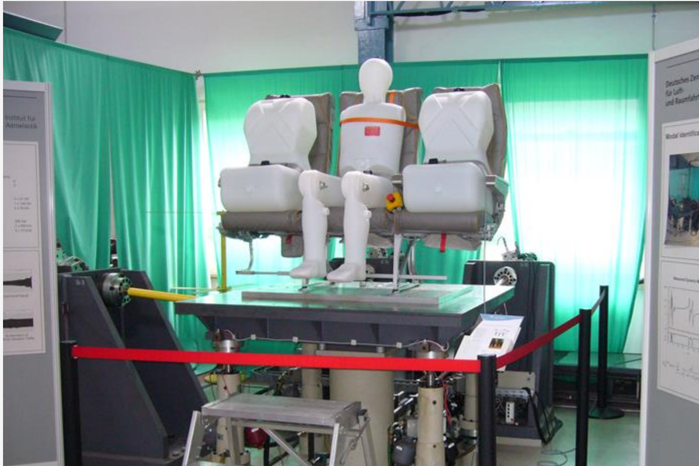
German Aerospace Center (DLR), Göttingen: Multi-axis vibration testing at the Institute for Aeroelasticity
