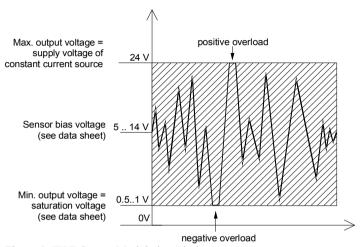
Figure 5: IEPE Sensor Modulation Limits
