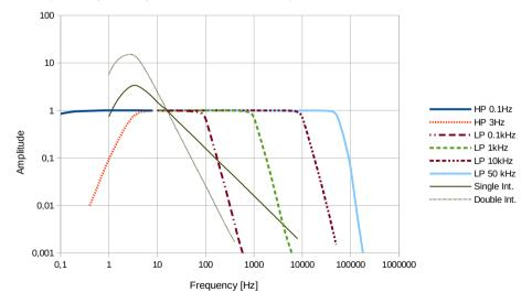
Figure 6: Frequency Response of the Filters and Integrators
