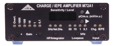
Figure 1: M72A1 front panel
