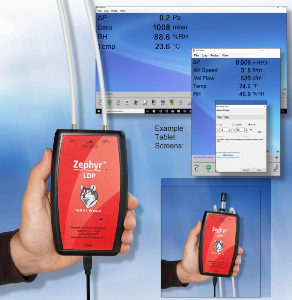
The GrayWolf Zephyr-LDP module, which connects to Windows tablets/ laptops/PCs for display and datalogging, has exceptional low-end accuracy, yet a wide range. Auto-ranging ΔP sensors combine with auto-zeroing for outstanding performance.
