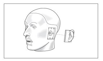
Standard pinnae are push mounted from the outside. The anthropometric pinnae, however, are secured from the inside by two screws in addition to the push mounting.
