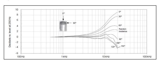
Free-field corrections for different angles of incidence
