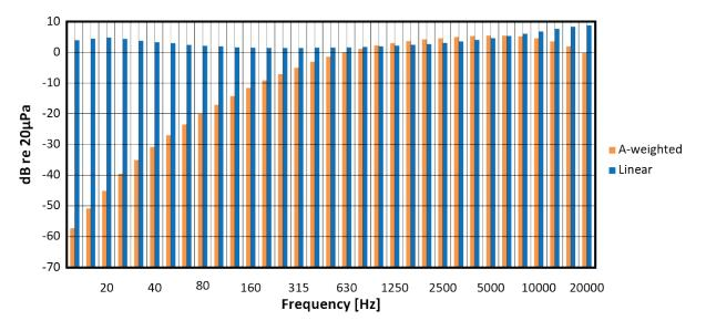
Typical noise floor in dB shown in 1/3-octave bands–linear and A-weighted.
