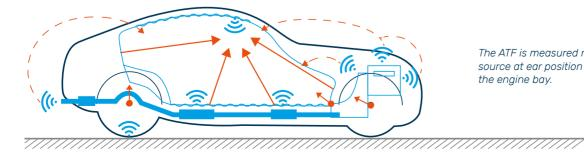
The ATF is measured reciprocally with a noise source at ear position and the response in the engine bay.
