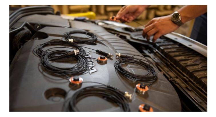
Since the 147AX operates in the -40 to 125 °C (-40 to 257 °F) temperature range and is designed to be water and dust proof (IP67), it will survive even the most challenging engine bay environments.
