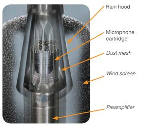
The microphone cartridge is protected by dust mesh, rain hood, windscreen and desiccator to obtain Ingress Protection Category IP55 according to IEC 60529.
