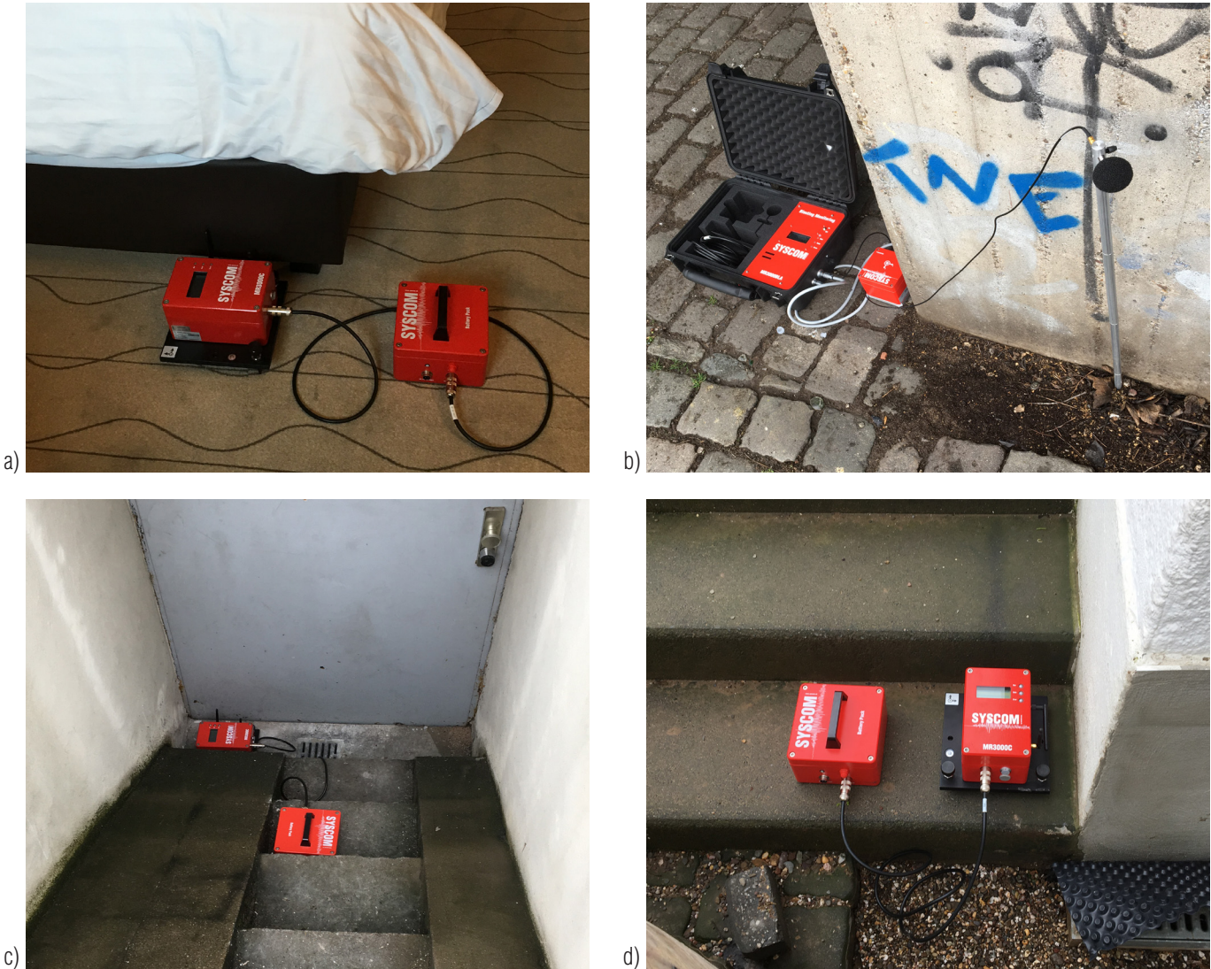
Figure 3. Instruments installed for the vibration monitoring: MR3000C in MP1 (a); MR3000BLA in MP2 (b), MR3000C in MP3 (c) and MR3000C in MP4 (d).
