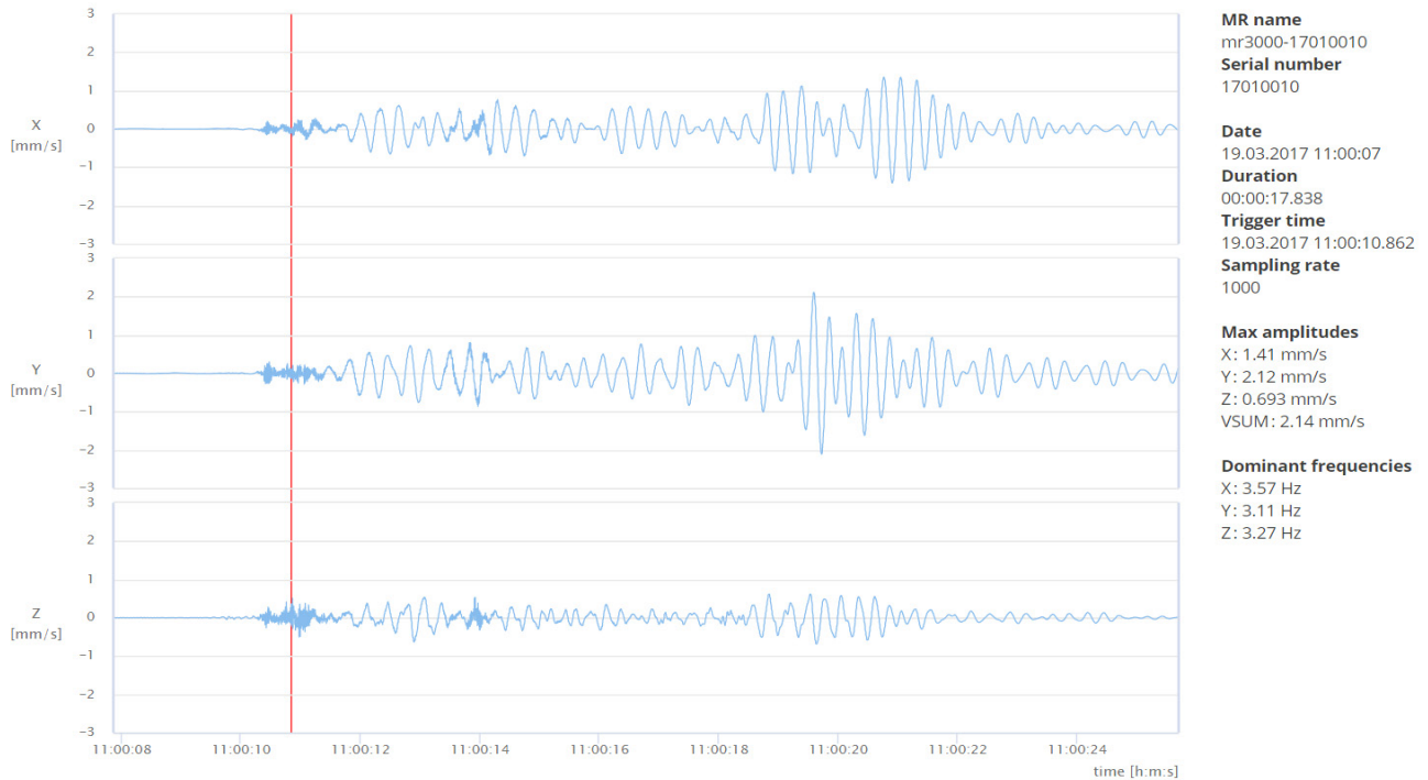
Figure 5. Time histories recorded in MP1, in the Bonn Marriott Conference Hotel, during the demolition of the Bonn Center.
