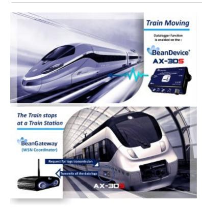
• In standalone operation, the BeanDevice® AX-3DS stores all the measurements on its embedded datalogger. Thus, a direct connection with the BeanGateway® is not needed.
