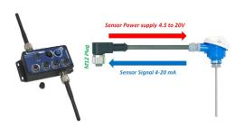
The sensor is directly powered by a high accuracy and adjustable DC/ DC converter integrated inside the device. The excitation voltage is remotely configurable through the BeanScape® (4.5 to 20V).
