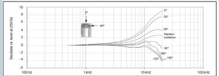
Free-field corrections for different angles of incidence
