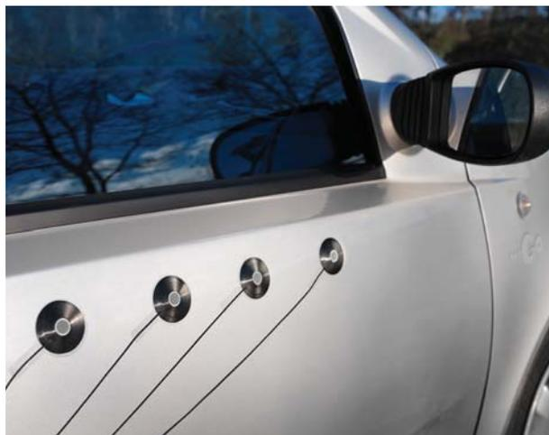
*Fig. 3 An array of four Surface Microphones mounted on the external surface of a car*
