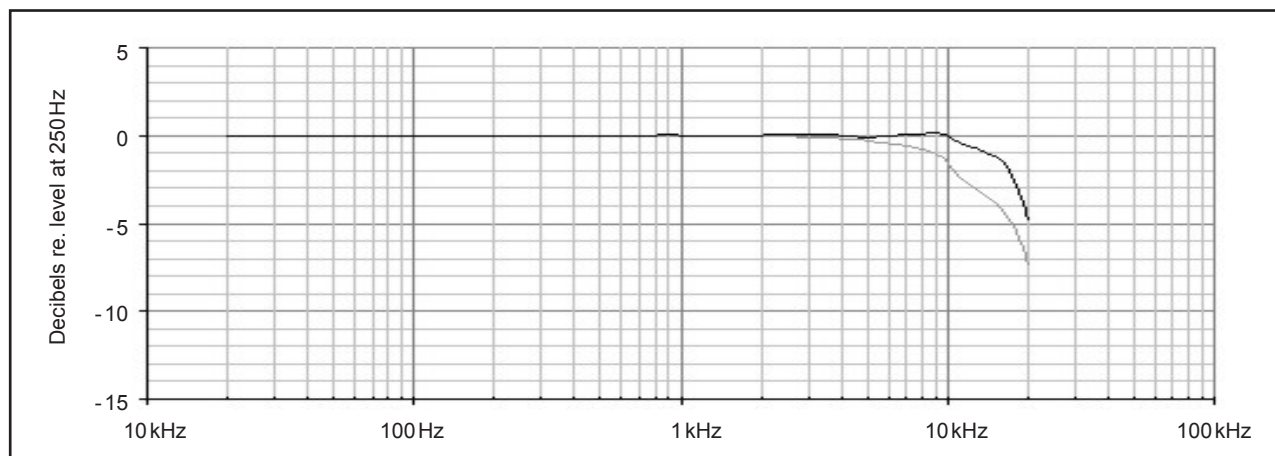
Fig. 2 Typical frequency response for Type 40AR. Upper curve shows response in a diffuse sound field (random incidence), lower curve shows pressure response
