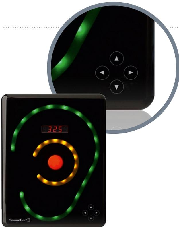
Located on the front of SoundEar®3 you will find a touch display from which you can control the device manually.
