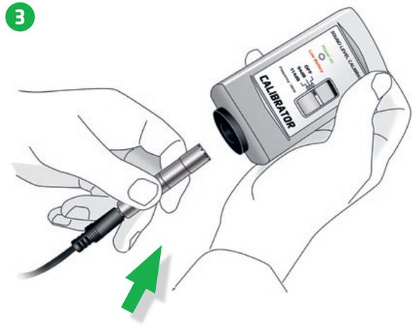
Set the calibrator to 94 dB and connect the microphone.
