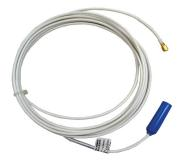
For probe lengths not listed, double the probe's desired physical length in inches and substract from 180 in. for a 15 ft. system or from 240 in. for a 20 ft. system to get the correct extension cable length.
