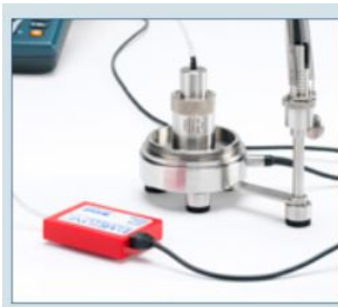
Type 43AB – IEC 60318-5 Reference Coupler (2cc) shown with insert earphone 3A
